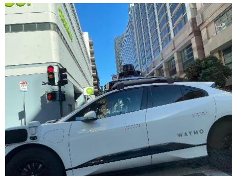
Figure 2. Self-driving taxi using LiDAR system (source: photo taken by the authors)
